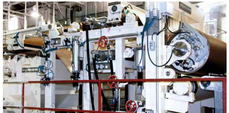
Newly designed sheeting machine for even higher outputs and optimised process control
