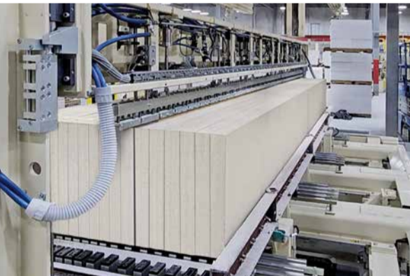
Precise AAC panel separation requires the right machine – delivering precise, smooth and marketable results.
