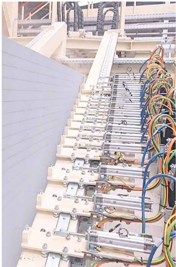
The uniform distribution of the wires minimises stress and ensures maximum cutting accuracy with automatic wire adjustment.
