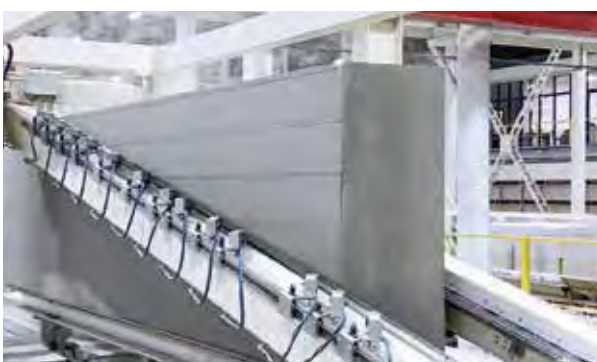
Uniform distribution of cutting wires reduces stress during thickness cutting
