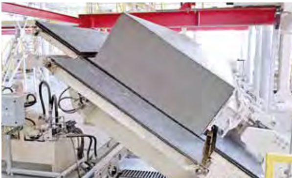
Tilt cake cutting: less binders and shorter precurving times
