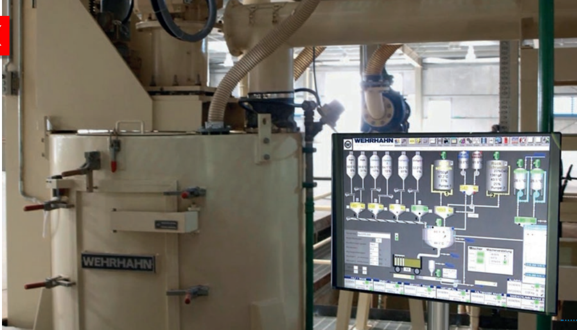
Graphical symbols on the operator screen give a clear overview of the AAC dosing process
