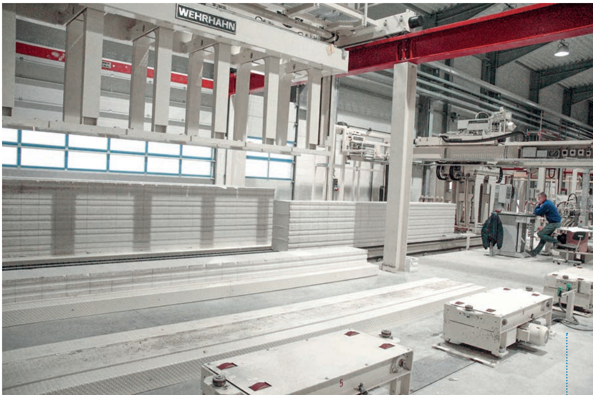
Fully automatic process: smooth production, consistent product quality, relaxed operators.
