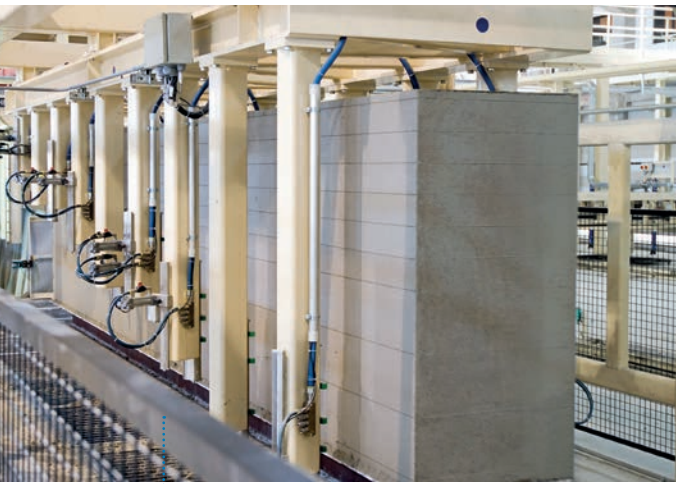
Before (left) and after (right) modernisation. From precise to utmost precision and flexibility: new thickness cutter with automatic wire adjustment
